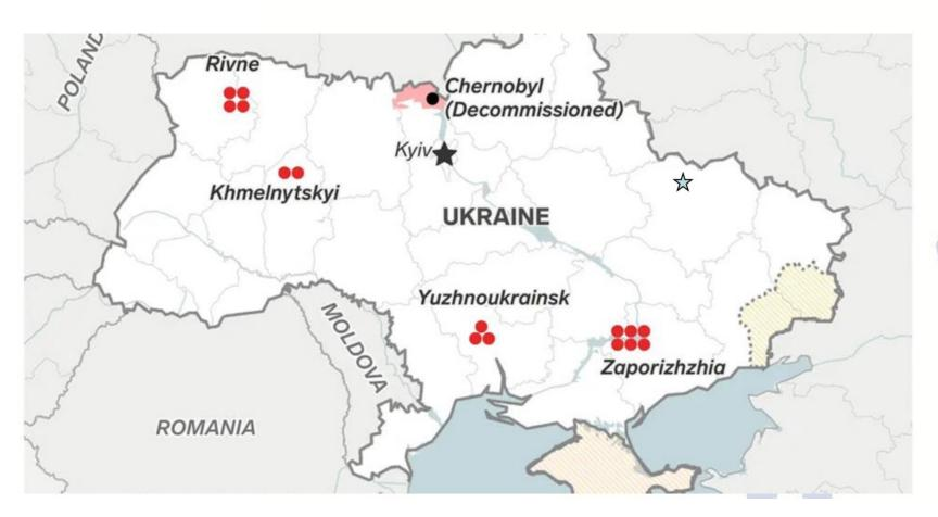
15 operating NPPs in Ukraine on 4 sites which are all Russian designed VVER types (mostly 1000 MW). The VVER NPPs in Ukraine are relatively modern (mainly built in the 1980s and 1990s) and are water cooled and water moderated.
